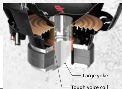
6-Layer Copper Voice Coil (Wire dia. 0.45mm) Aluminum Bobbin
