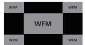
Display position selection: four corners and large center, with adjustable transluence
