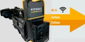
The SpeedFusion Engine Cam (SFE Cam) uses SpeedFusion bandwidth bonding technology to combine the reliability and bandwidth of two cellular connections and Wi-Fi, giving you rock solid data link for live streaming\*. With redundant SIM slots, the SFE Cam gives you a total of four SIM cards to select from. WAN Smoothing and FEC protect your video stream from the effects of packet loss.
