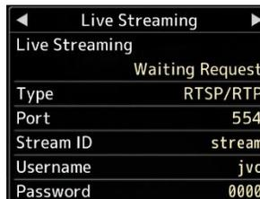
8. From Tricaster Mini Dashboard, click NET1 to RECEIVE. Stream should appear as NET1 input. Live Streaming should change from Waiting Request to In Progress.
