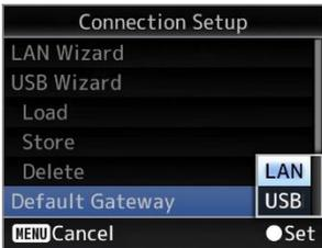
4. Click on Menu > Live Streaming Set. Scroll down to Interface. Select the correct Interface depending on network connection.
